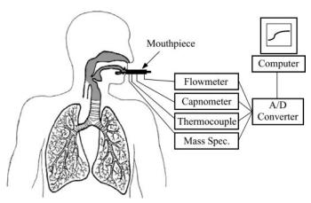
Fig. 1. Schematic of experimental setup. A linear resistance attached to the end of the mouthpiece and a display of their exhaled flow rate on the computer monitor helped subjects maintain a constant exhaled flow rate. Acetone concentration was measured by using the mass spectrometer. A/D, analog to digital
