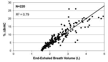
Fig. 5. %Change in breath alcohol concentration (BrAC) between the minimum (V = 1.5 liters) volume and end-expired volume increased with end-expired breath volume. A best-fit line shows a strong relationship between factors ( $r^2 = 0.79$ ).
